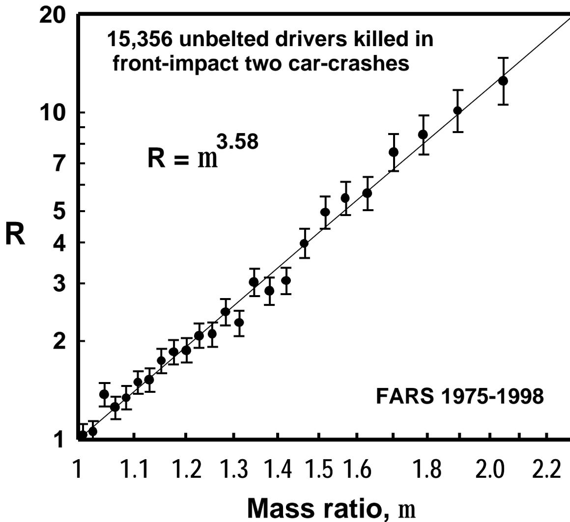
FIGURE 1 The ratio, R, of driver fatalities in the lighter compared to in the heavier car versus the ratio,  $\mu$ , of the mass of the heavier to the mass of the lighter car for frontal crashes (both cars with principal impact point at 11, 12 or 1 o'clock). The relationship is the first of the two “laws” of two-car crashes.
