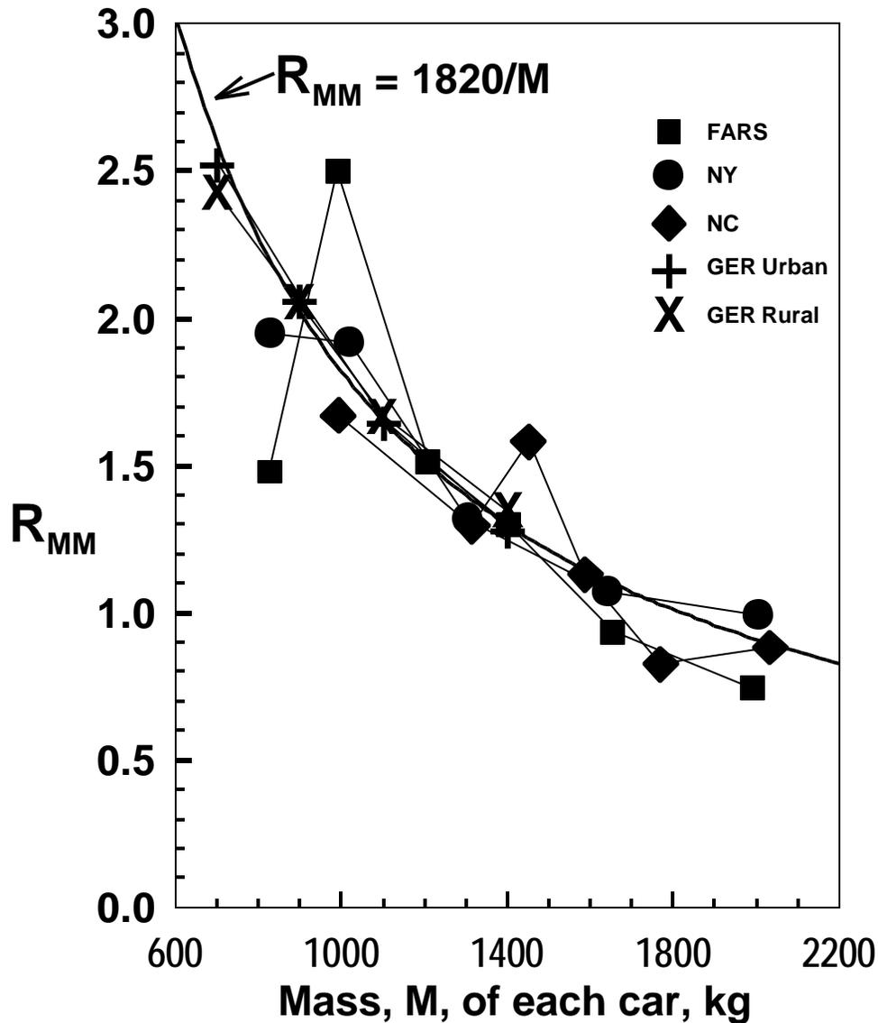
FIGURE 2 Relative risk,  $R_{MM}$ , of driver injury or fatality when cars of similar mass crash head-on into each other versus  $M$ , the mass of each car. In all cases the data are scaled to assign a risk of 1.3 to  $M=1400$  kg. The relationship is the second of the two “laws”.
