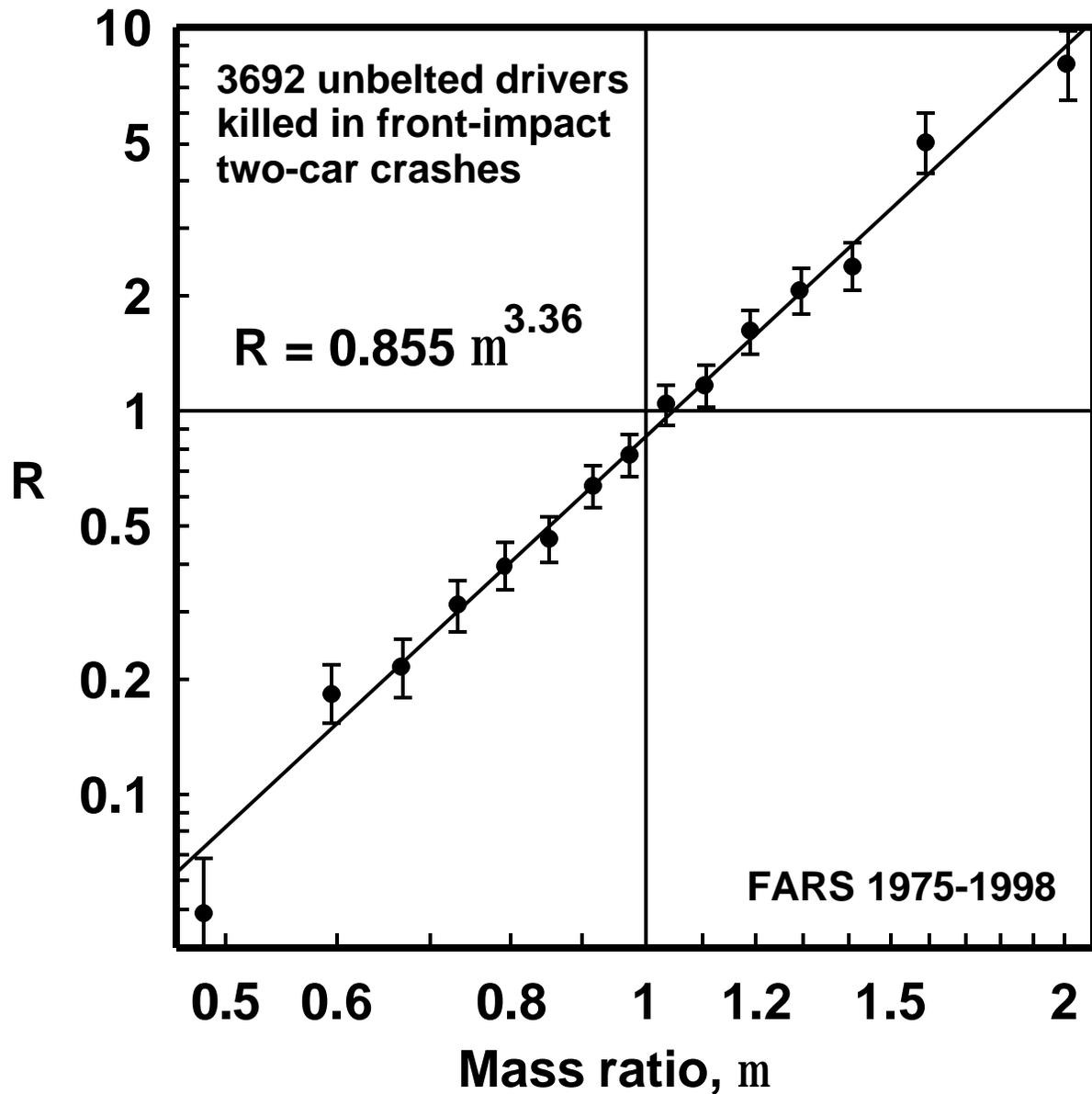
FIGURE 3. The ratio, R, defined as the number of accompanied drivers killed divided by the number of lone drivers killed in the same crashes, versus  $\mu$ , the curb mass of the lone drivers' cars divided by the curb mass of the accompanied drivers' cars. When the cars are of equal mass, the presence of a passenger is associated with a change in R of -14.5%.
